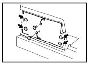
2 Dust off the surface of the CCD Filter by using a blower brush or a piece of soft cloth.
